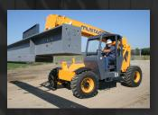
Pilot-assisted joystick controls for boom, fork tilt and frame level functions are easyto-operate, reducing operator fatigue.
